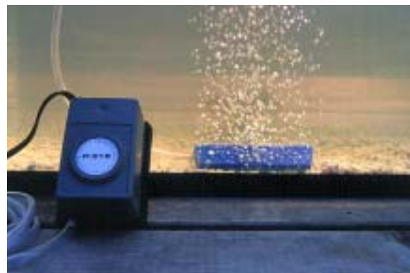
Many medications require ample aeration of the water. An aerator pump affixed to a bar air-stone provides this.
