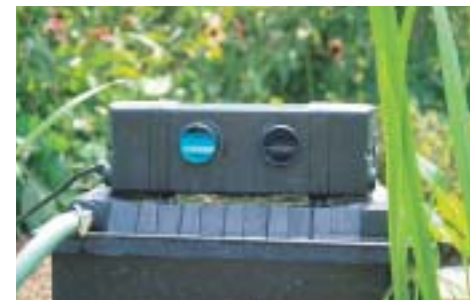
Ultraviolet Clarifier Unit
